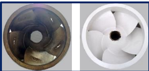
Application of ceramic putty on fan blades
