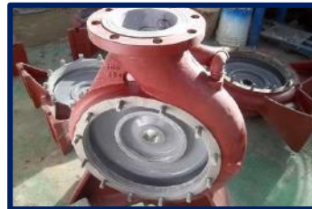
Application of ceramic putty on pump housing
