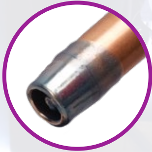
WITH ANTI SPATTER PASTE BEFORE WELDING
