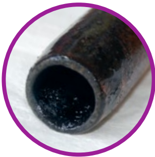
WITH ANTI SPATTER PASTE, AFTER WELDING
